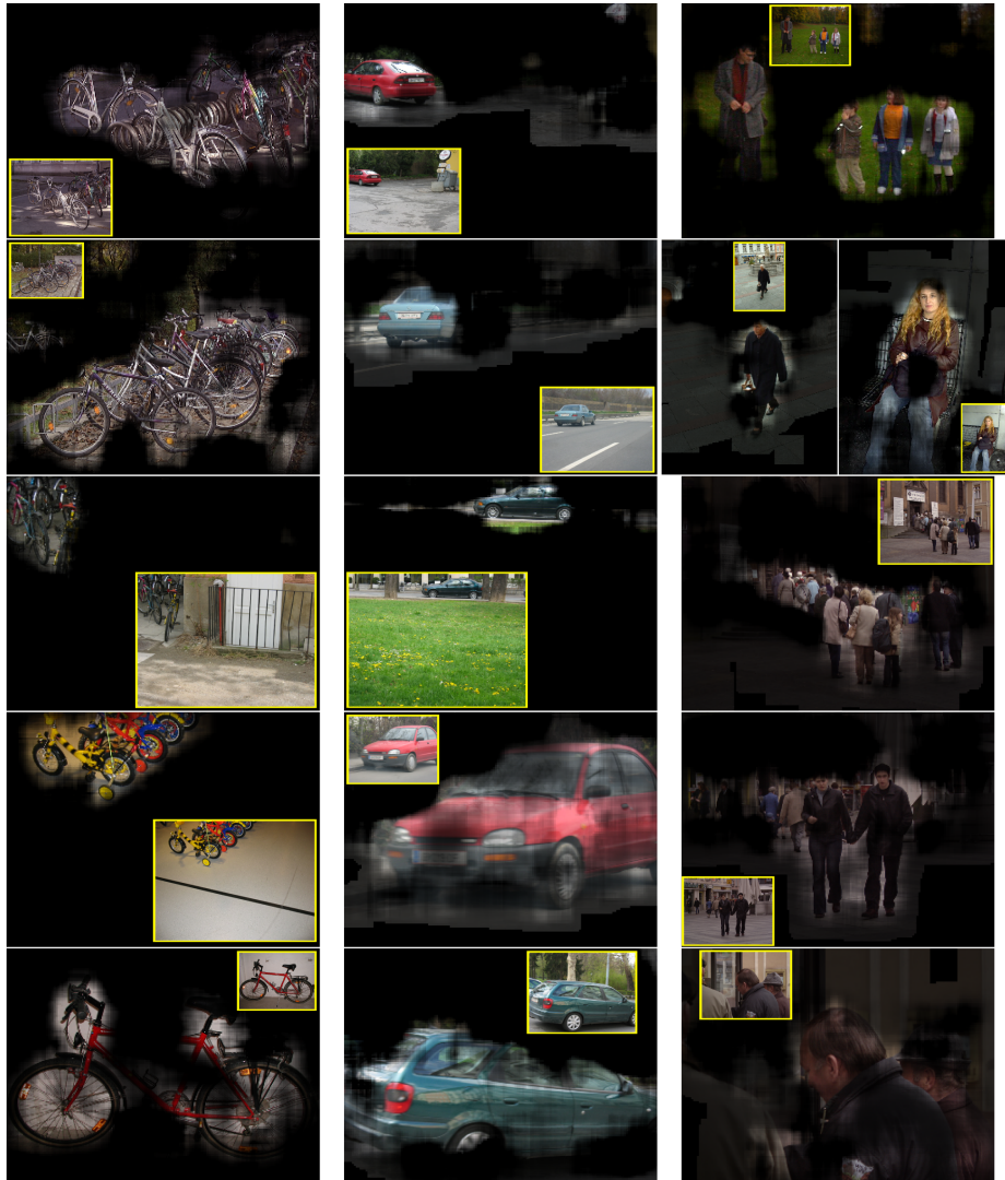
Fig. 4. Selected results on Graz-02. (Best viewed in color). Images are first masked by the classification then transformed to HSV. The HSV images have their V channel weighted by the confidence in the classification, darkening the pixels which are less confident about the class. All images shown were generated with the parameter set denoted AIB200RGB and classified with an SVM.
