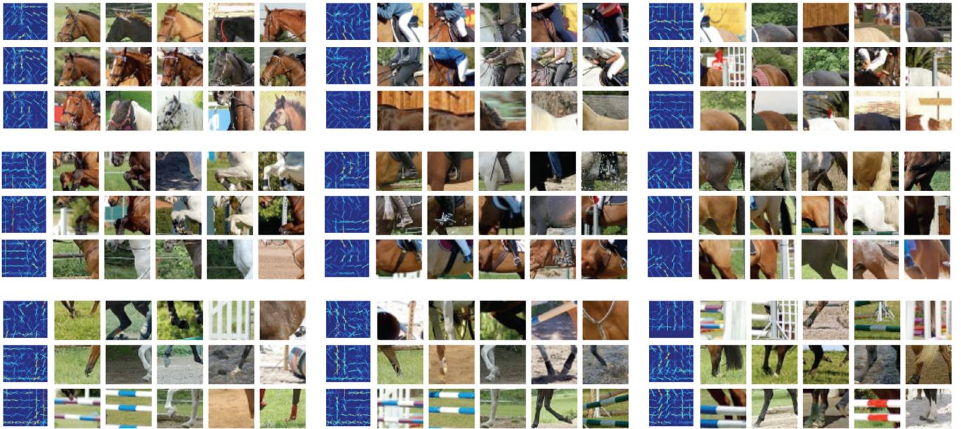
Fig. 8. Top scoring detection for each appearance of each part the class horse. Note the differences that we capture in the appearance of the head and the legs, or in the rider.
