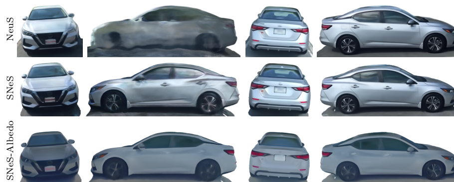
Fig. 5. Novel view renderings of the partly-observed (left) and fully-observed (right) sides. Top row: NeuS. Middle row: SNeS. Bottom row: SNeS albedo maps.
