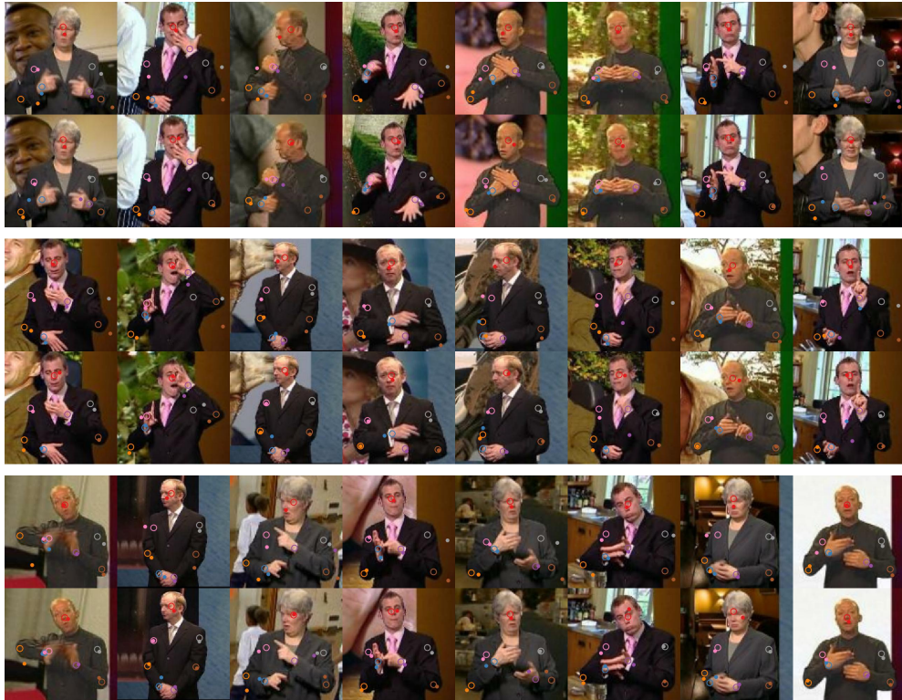
Figure 3: Learning Human Pose. 50 unsupervised keypoints are learnt. Annotations (empty circles) for 7 keypoints are provided, corresponding to — head, wrists, elbows and shoulders. Solid circles represent the predicted positions; Top rows show raw discovered keypoints which correspond maximally to each annotation; bottom rows show linearly regressed points from the discovered keypoints. [above]: randomly sampled frames for different actors [below]: frames from a video track.
