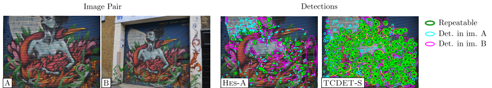
Figure 4: Example of an image pair where a trained detector ( rep(\text{TCDET-S}) = 69.8 ) achieves better performance compared to a traditional detector ( rep(\text{HES-A}) = 28.57 ).
