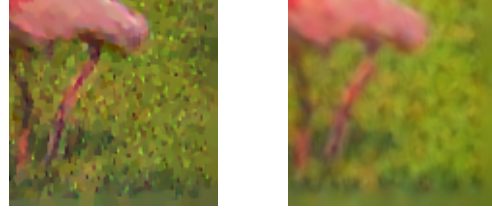
Figure 2. Left: Spikes in a inverse of norm1 features - detail shown. Right: Spikes removed by a V^\beta regulariser with \beta = 2 .
