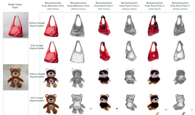
Figure 9. Effect of normal smoothness on reconstruction quality. Each pair of rows show the reconstruction without and with the normal smoothness regularization term (4). The regularizer improves the visual appearance of surfaces and reduces the number of irregularities on the surface of reconstructed objects. In most cases, we also find that it helps to improve the overall realism of the reconstructed shape.
