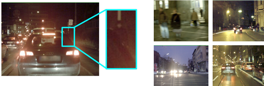
Fig. 1: Sample images from the NightOwls dataset exhibiting the challenges of detection at night. Occlusion, low contrast, motion blur, image noise and inhomogeneous illumination (left) and different illumination and weather conditions (right).
