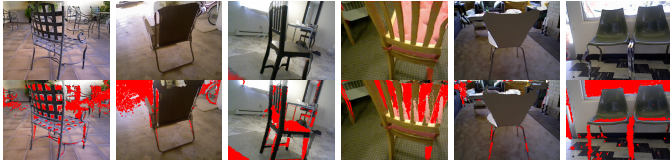
Fig. 7. Data augmentation. Training samples generated leveraging monocular depth estimation ( ours , top) and using depth from ORB-slam2 (baseline, bottom). Missing pixels due to missing depth in red.
