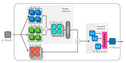
Figure 2: **Trajectory attention flowchart.** We divide the attention operation into two stages: the first forming a set of ST trajectory tokens for every space-time location st—a spatial attention operation between pairs of frames—and the second pooling along these trajectories with a 1D temporal attention operation. In this way, we accumulate information along the motion paths of objects in the video. The softmax operations are computed over the last dimension.
