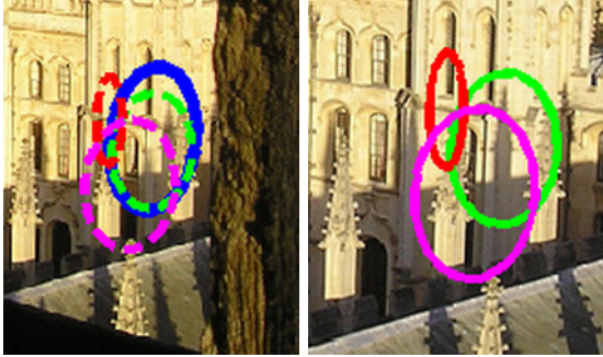
Fig. 2. A close-up of a pair of reference (left) and target (right) images from the Oxford5K dataset. A feature region in the reference image is shown with solid blue. Its putative positive, negative, and ambiguous matches in the target image are shown on the right with green, red, and magenta respectively. Their projections to the reference image are shown on the left with dashed lines of the same colour. The corresponding overlap ratios (with the blue reference region ellipse) are: 0.74 for positive, 0.04 for negative, and 0.33 for ambiguous matches.
