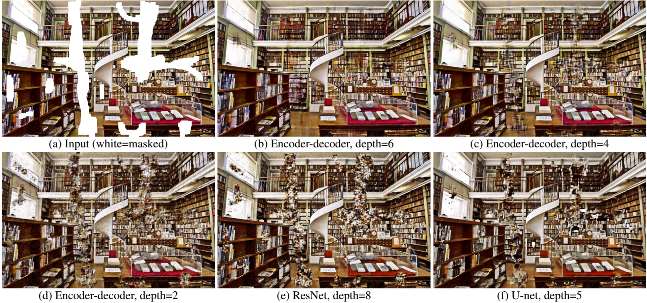
Figure 8: Inpainting using different depths and architectures. The figure shows that much better inpainting results can be obtained by using deeper random networks. However, adding skip connections to ResNet in U-Net is highly detrimental.
