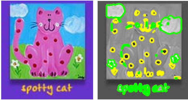
Figure 2: MSER. Left: original image. Right: detected MSER regions (green: positive level sets, yellow: negative level sets).
