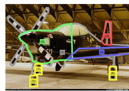
airliner: no; is-cargo-plane: no; is-glider: no; is-military-plane: yes; is-propellor-plane: yes; is-seaplane: no; plane-location: on ground/water; plane-size: medium plane; wing-type: single wing plane; undercarriage-arrangement: one-front-two-back; airline: UK-Air Force; model: Short S-312 Tucano T1 2 vertical stabilizer tail-has-engine: no-engine nose has-engine-or-sensor:
